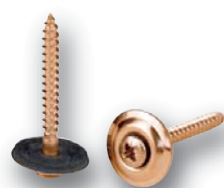
Raised countersunk head wood screws with sealing washer 19mm Material: stainless steel A2 (AISI 304) copper plated
