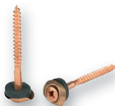
Raised countersunk head wood screws with sealing washer 15mm Material: stainless steel A2 (AISI 304) copper plated
